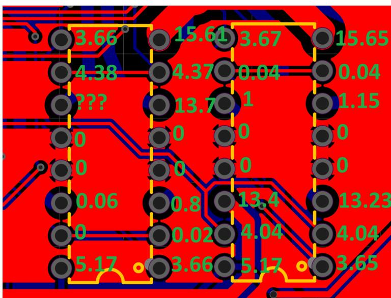
Fried an Arduino because I shortened the ??? pin with the neighboring digital pin of the Arduino. The voltage there should be around 13.7V
