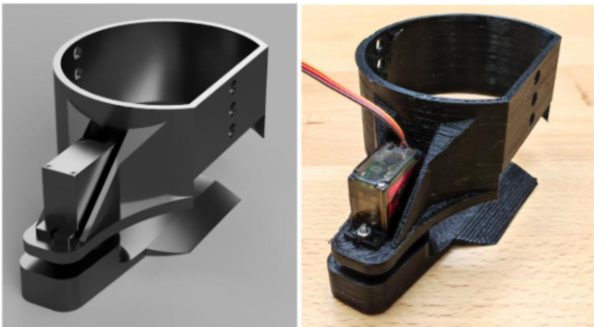
After some tweaking, this approach is also able to pick up the rescue kit reliably, as the wedge causes the kit to rotate. Gravity then does all the work for us, tipping over the kit onto the wedge
