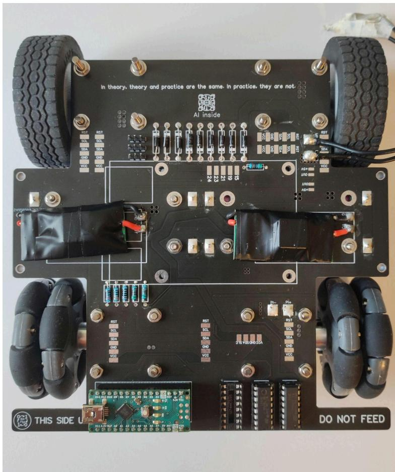
Working so far, but the right side turns slower than the left side. Voltage left: 12V, voltage right: 11.6V
