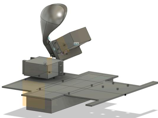
Problem: as the gripping mechanism is quite high (causing the overall camera height to increase as well), we decided to move the whole mechanism a bit to one side:
