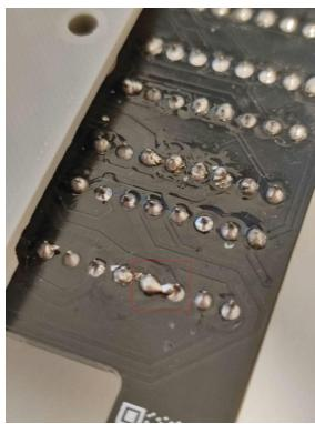
The output of the motor was directly connected to GND causing a massive current flow. New problem: motors receive more than 12V, probably problem with duty cycle calculation
