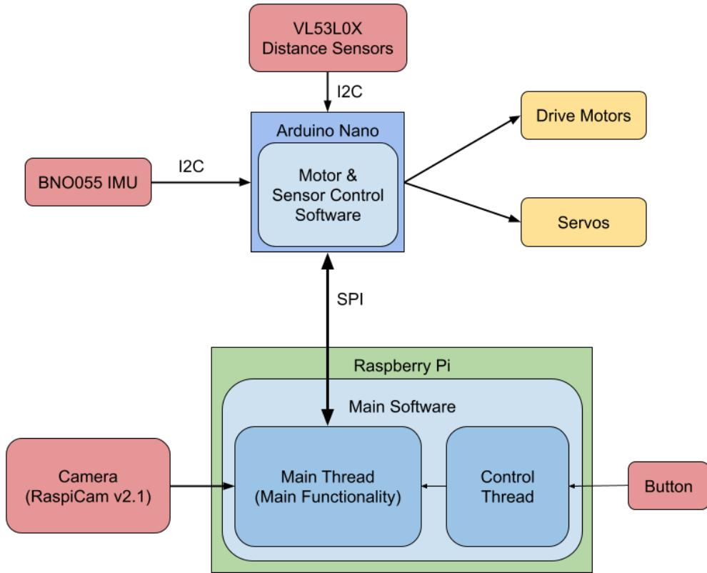
Differences to last year: SPI instead of UART over USB. Main software split into two threads (maybe more threads for obstacle, silver, etc. later). Control Thread now continuously monitors the button, this way the robot can be stopped at any time.
